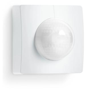
The IS 3180 DCS mounts on a wall and is designed to control a variety of building spaces. The sensor is part of the STEINEL family of high performance commercial occupancy sensors. IS 3180 DCS sensors are passive infrared and respond to heat radiated from human body motion. After a period of time where no occupancy has been detected, the sensor switches lighting OFF.
